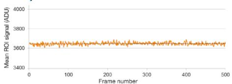
EM Gain stability in the iXon Ultra 897 @ 55 fps. 500 frame kinetic series; frame transfer (overlapped) acquisition; 17.8 ms exposure time; x300 EM gain.
